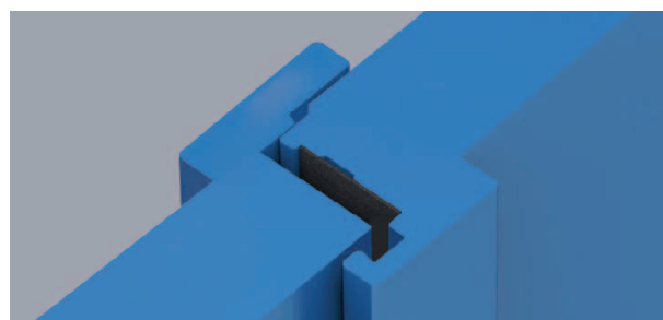
Horizontal cross section of the central rebate
